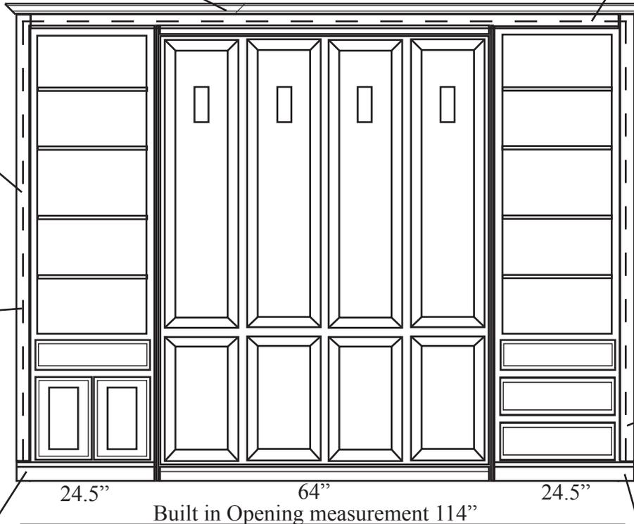
Cut base trim to fit space. This piece should be cut and attached first. Cut long enough to allow for the vertical trim piece to sit on top of the base trim.
