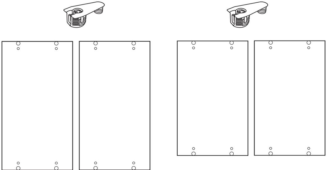
**Step: 6** Insert connecting bolts into the top four holes on the inside partitions as shown.
