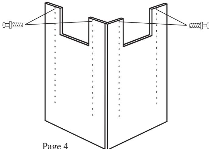
**Step: 7** Insert connecting bolts as desired for shelf height on the left and right sides. The connecting bolts placement must match so shelves will be level.
