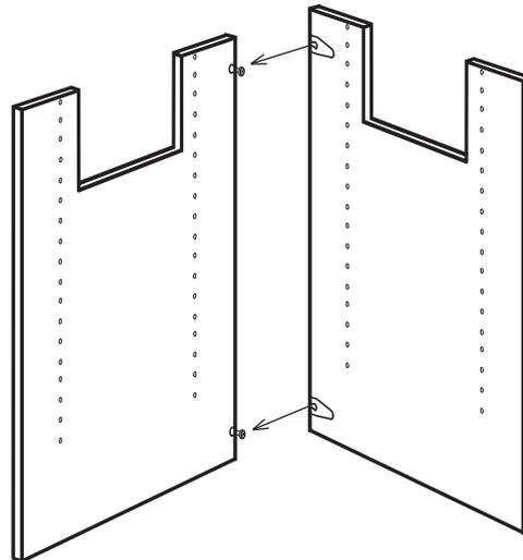
**Step: 4** Locate the two end partitions and insert connecting bolts in the top two holes as illustrated.
