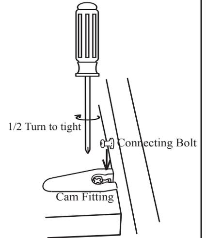
Step: 3 Using the cam fittings, connect the two partitions together as illustrated.
