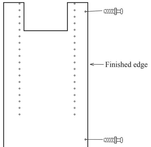
Step: 2 In the second partition, insert two white cam fittings into the sockets as illustrated. Verify the cam fittings are seated down firmly into the partition.
